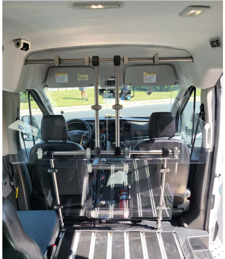
Full barrier which includes a sliding window for passenger interaction
